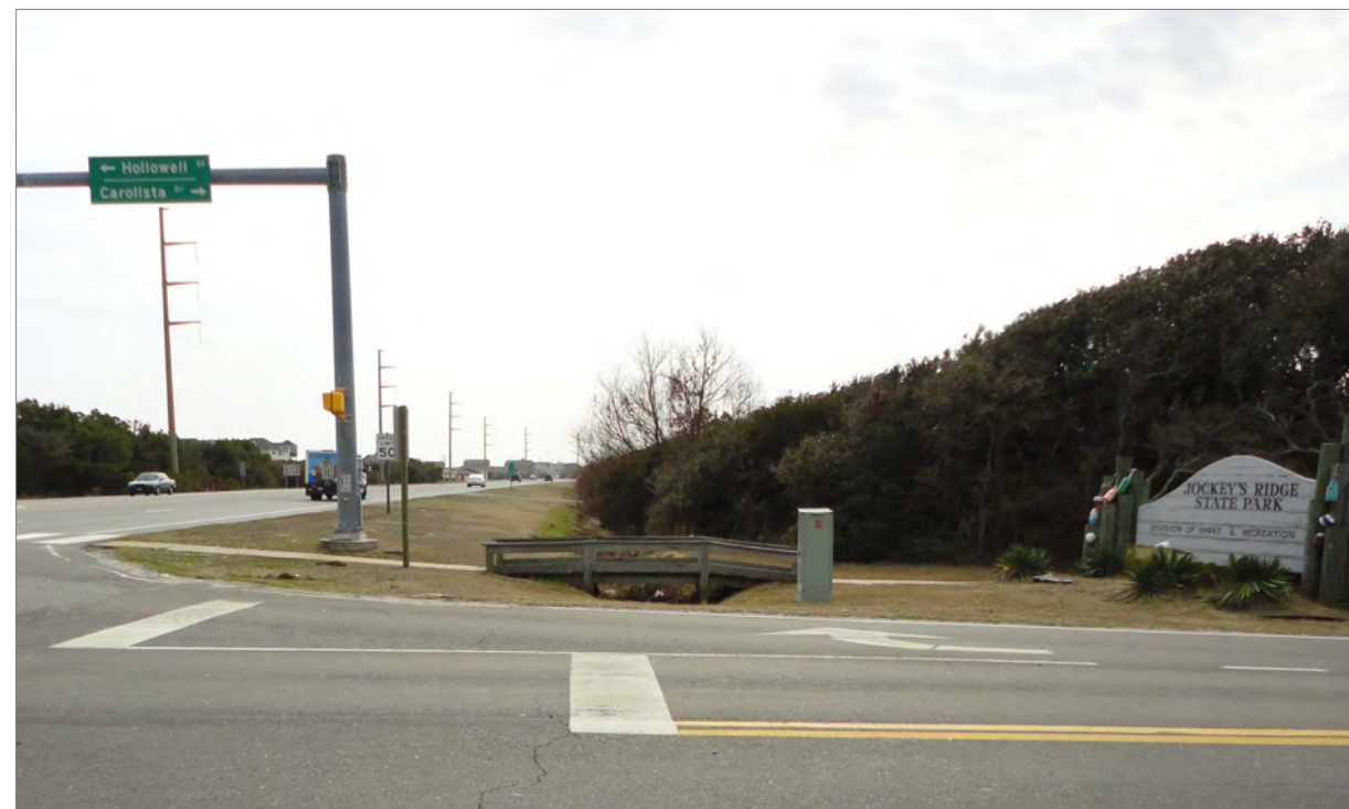
Looking south along US 158 from Carolista/Hollowell. The future path run between US 158 and the trees/vegetation shown in this photo. Crossing improvements would include high-visibility crosswalks and countdown signals for the trail.
